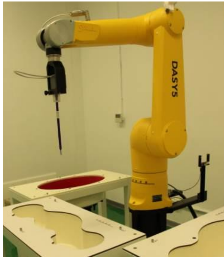
Picture D.6 DSY5 system Set-up
