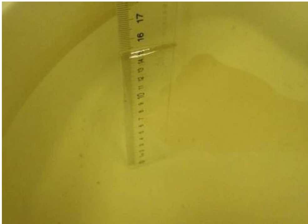
Picture 7.3 Liquid depth in the Flat Phantom (835MHz)
