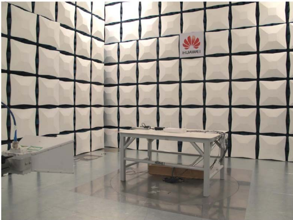
Radiated emission for 1GHz to 18GHz
