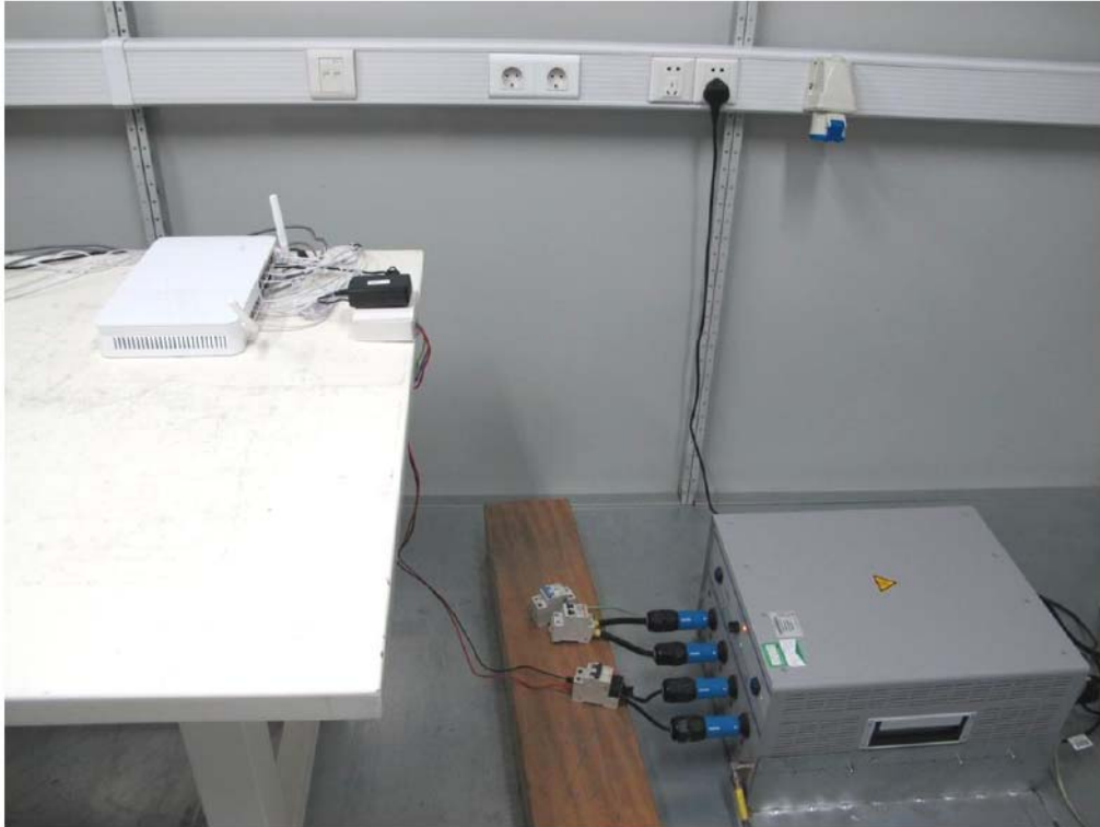
Conducted emissions of AC power port
