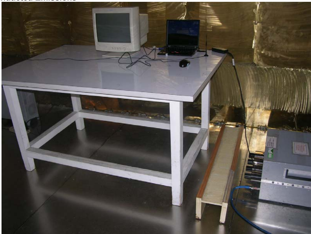
Conducted Emissions of AC Power Port
