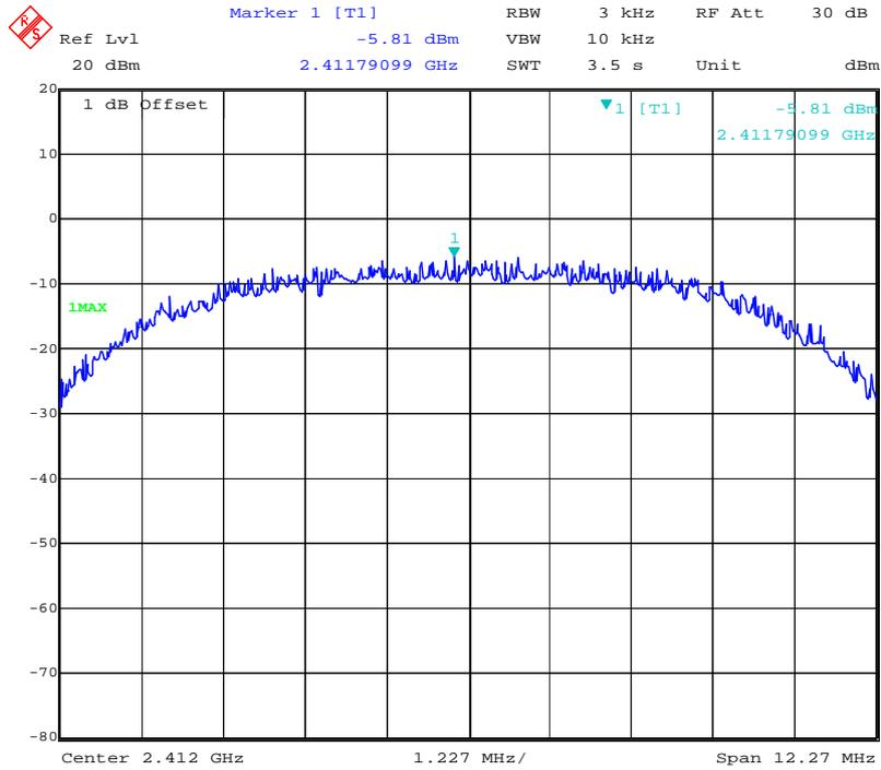
Power Spectral Density, 802.11b Middle Channel
