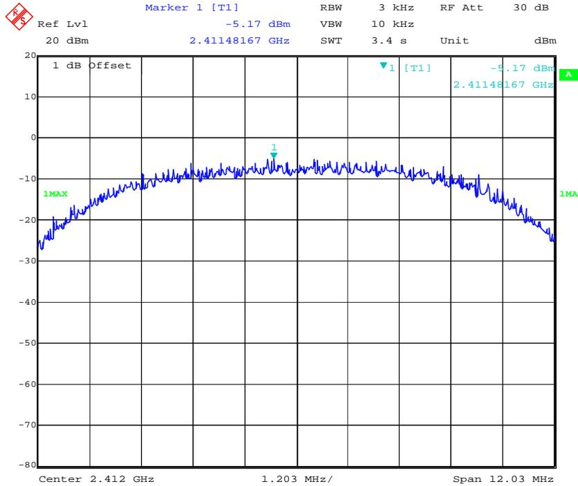
Power Spectral Density, 802.11b Middle Channel
