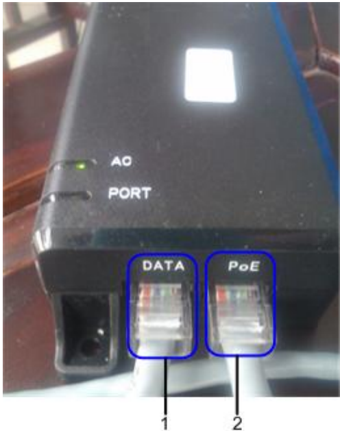
Figure 3-16 Connecting the PoE adapter
