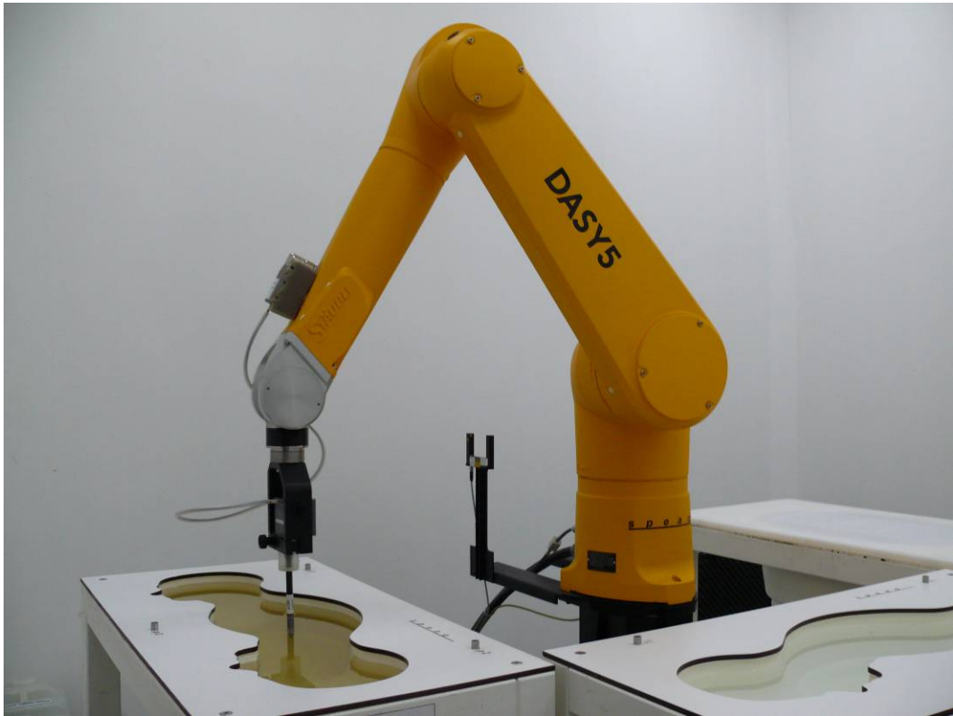
Picture 2: Specific Absorption Rate Test Layout
