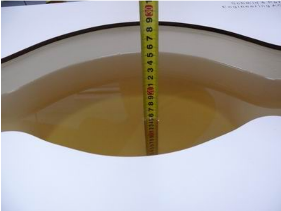
Picture 3: Liquid depth in the Flat Phantom (750 MHz, 15.3cm depth)
