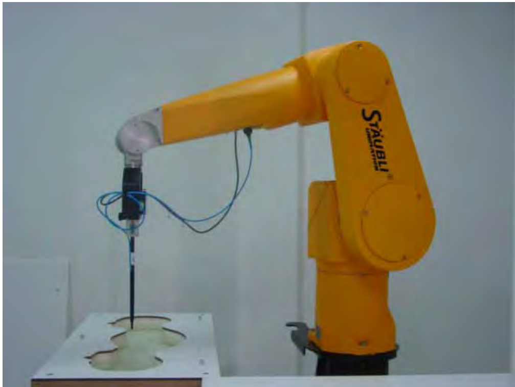
Picture B1: Specific Absorption Rate Test Layout
