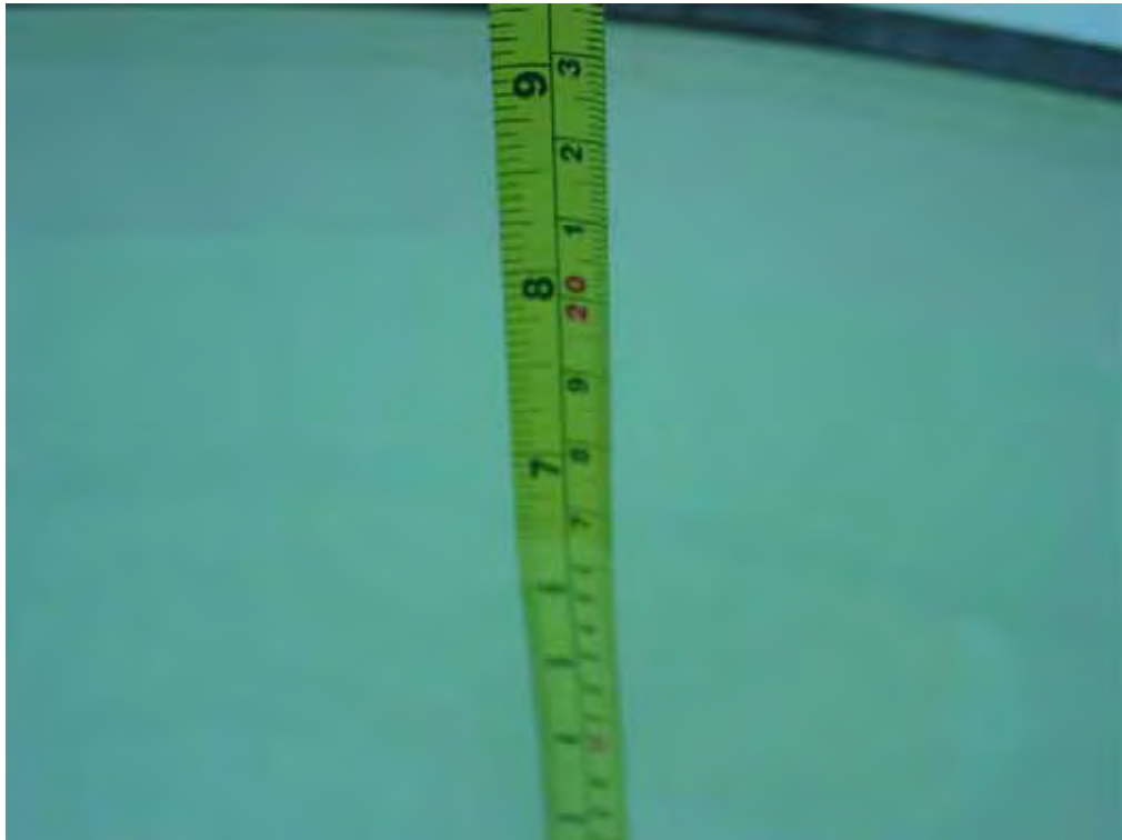
Picture B3 Liquid depth in the Flat Phantom (1900MHz)
