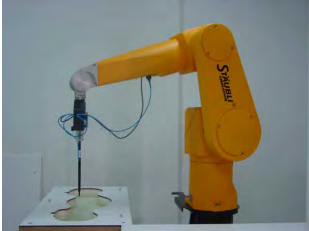
Picture B1: Specific Absorption Rate Test Layout
