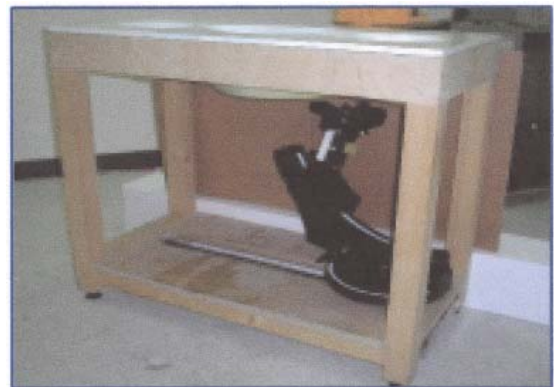
Picture 8: Generic Twin Phantom
