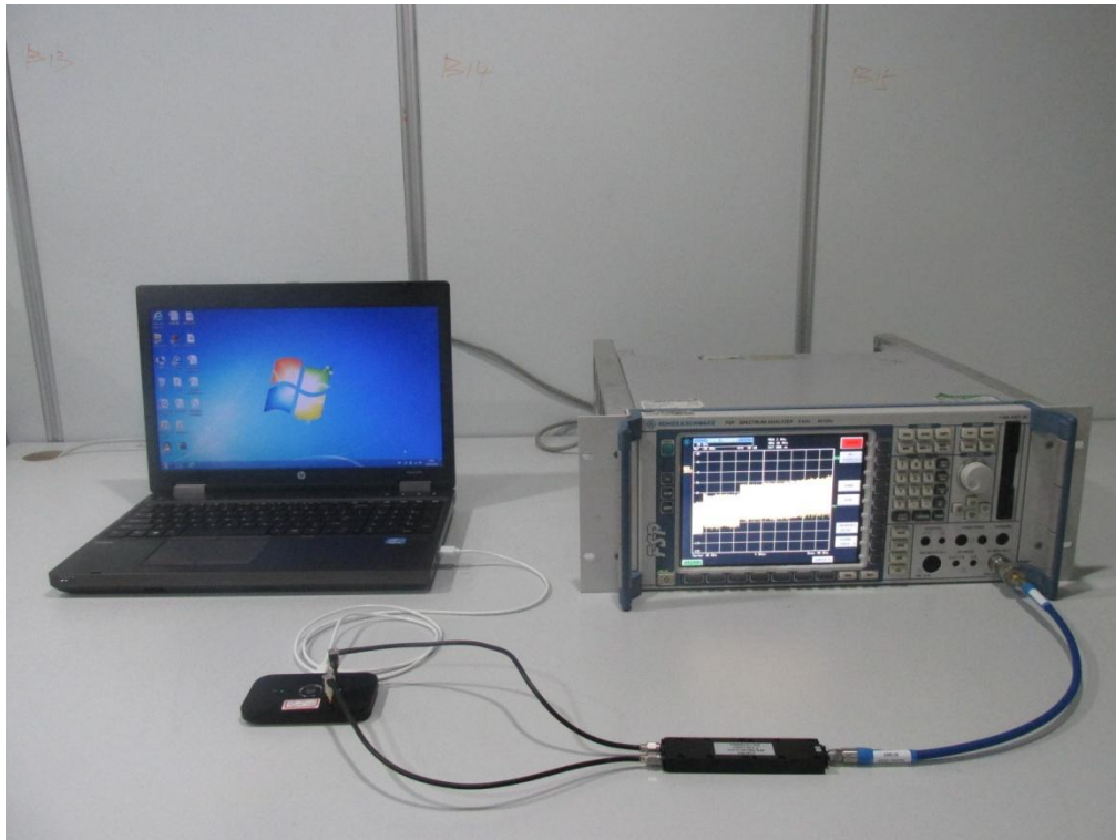
Conducted Test setup photo (MIMO)
