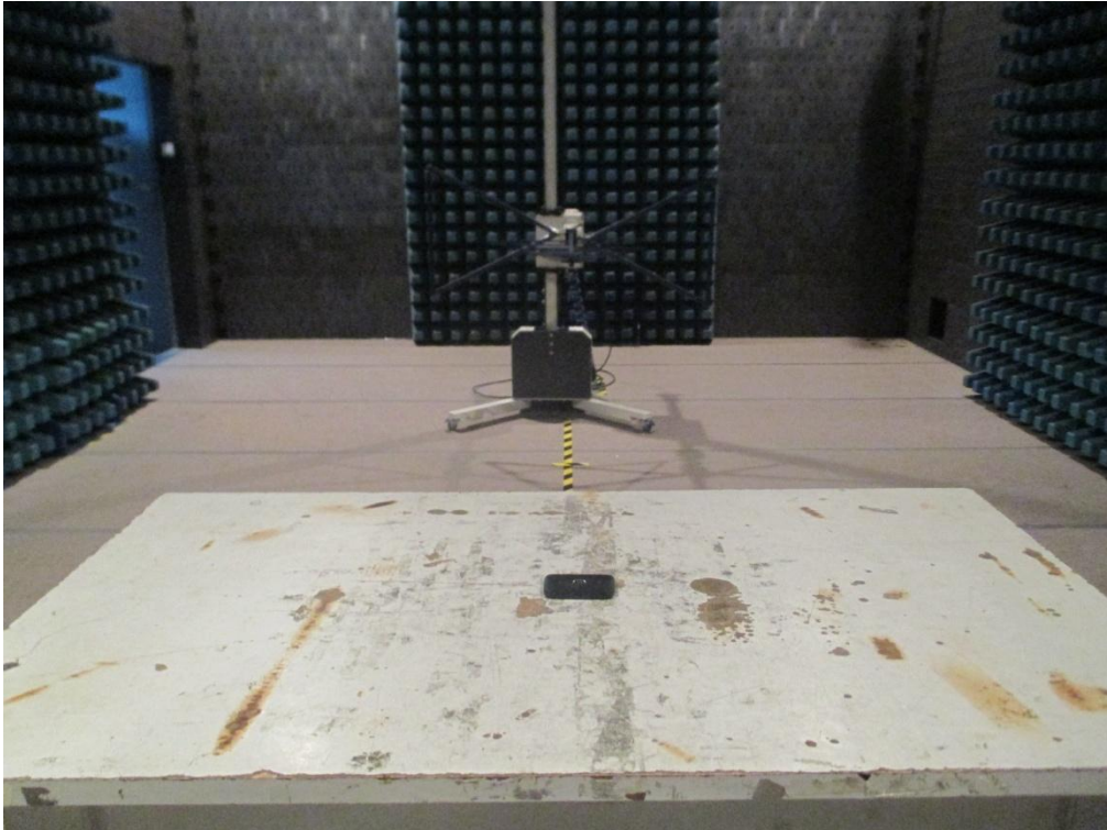
Radiated Emission Test setup photos
