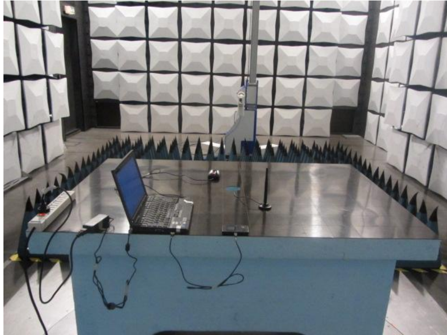
Radiated Spurious Emission (above 18GHz)
