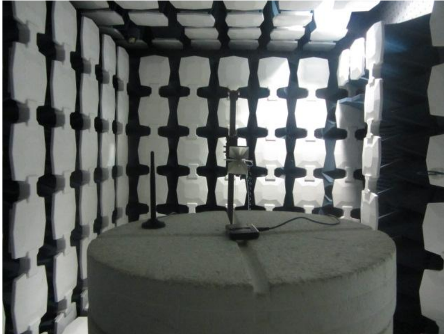
Radiated Spurious Emission (3GHz to18GHz)
