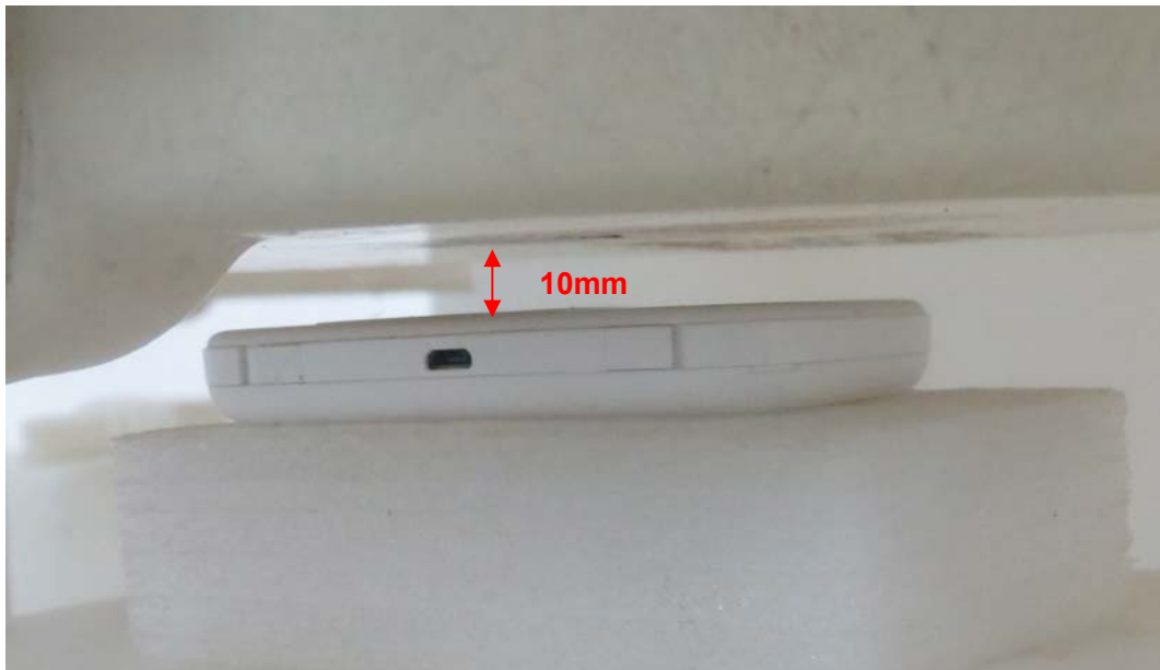
Picture 16: Test position 2 (Variant E5372s-32)
