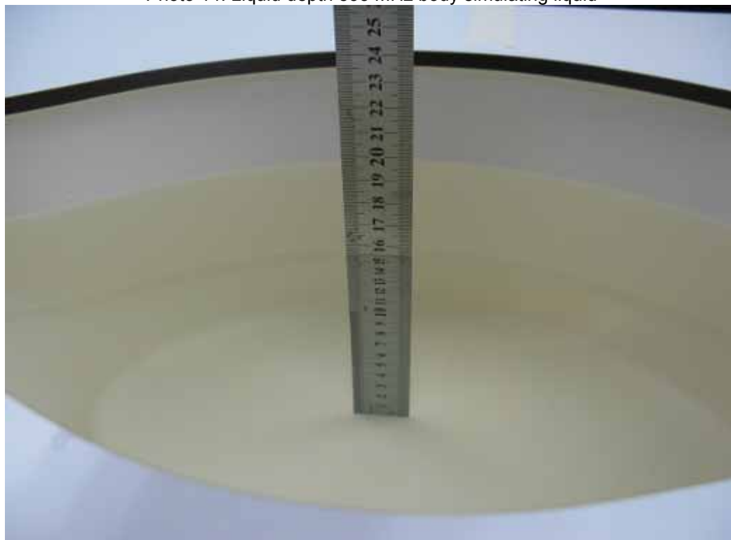
Photo 14: Liquid depth 835 MHz body simulating liquid
