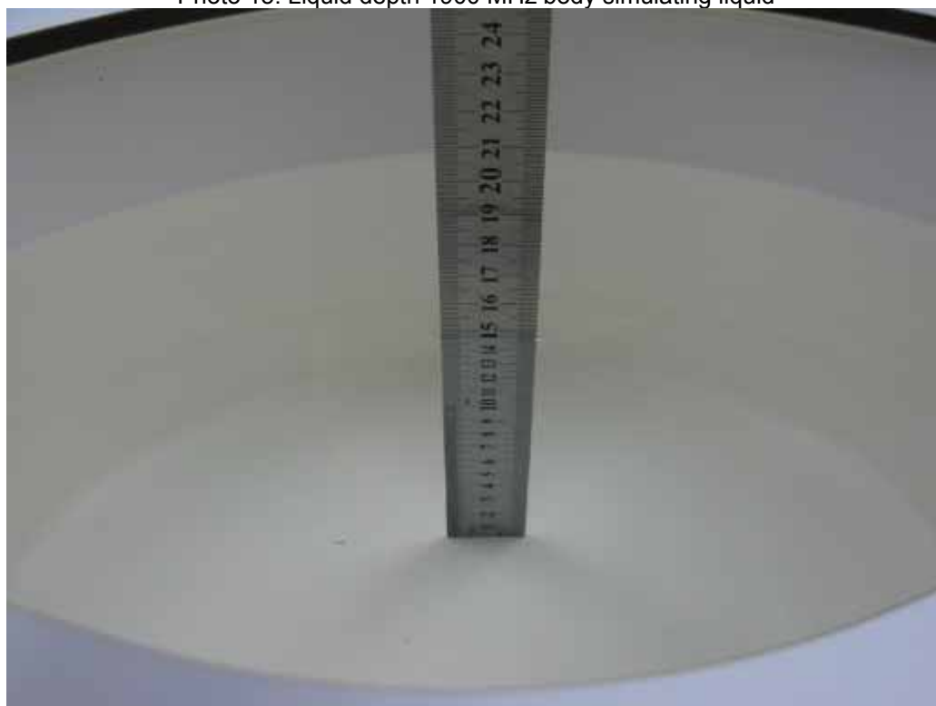
Photo 15: Liquid depth 1900 MHz body simulating liquid
