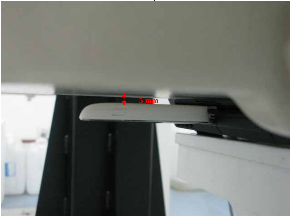
Photo 11: E367u-8 Test position of rear side
