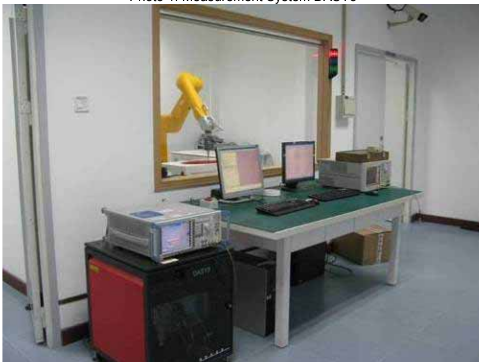
Photo 1: Measurement System DASY5
