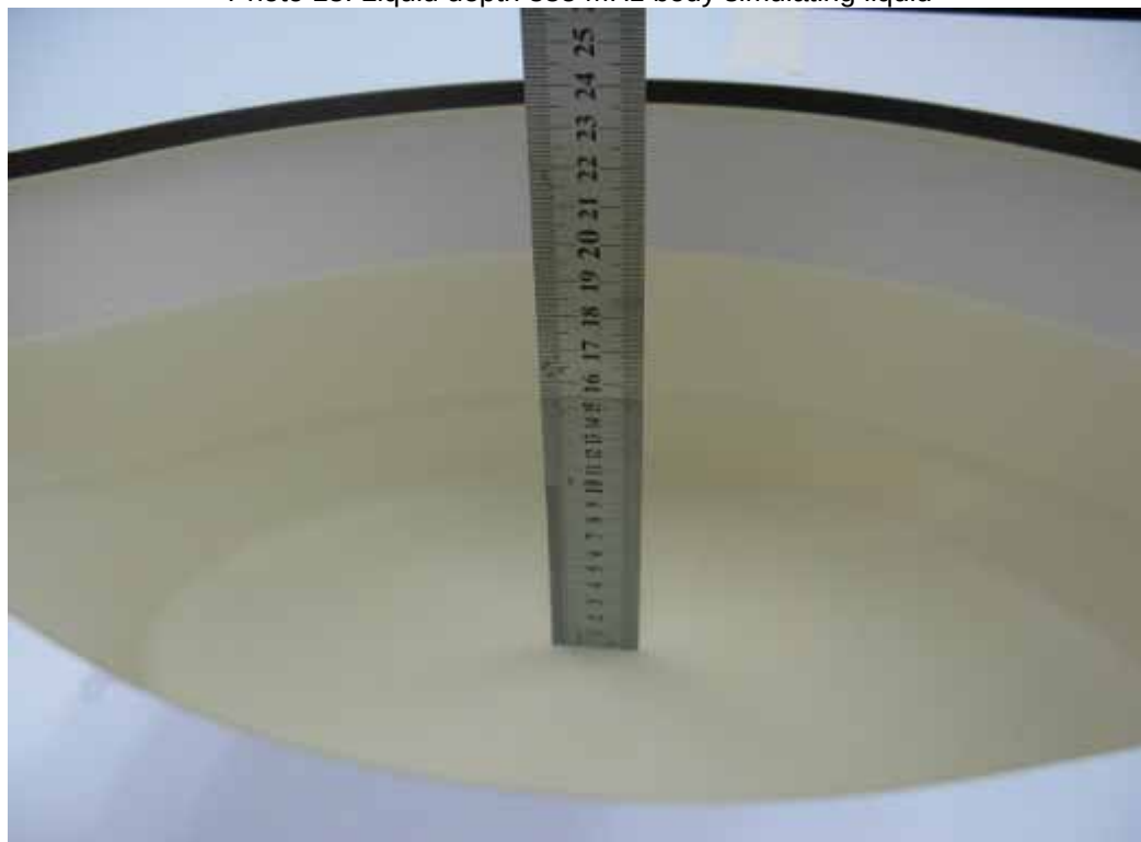
Photo 13: Liquid depth 835 MHz body simulating liquid
