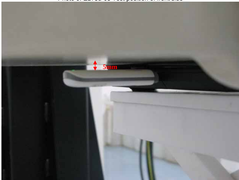
Photo 9: E173u-63 Test position of front side
