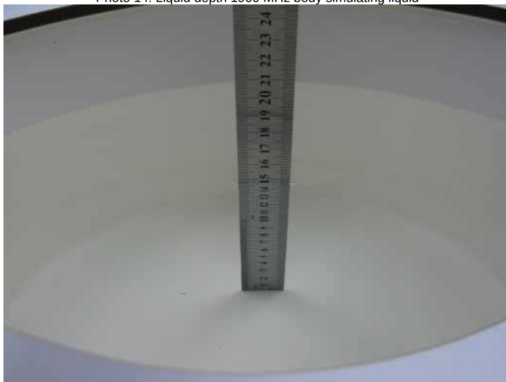
Photo 14: Liquid depth 1900 MHz body simulating liquid
