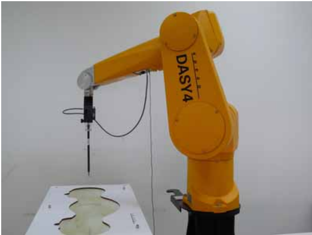
Picture 2: Specific Absorption Rate Test Layout
