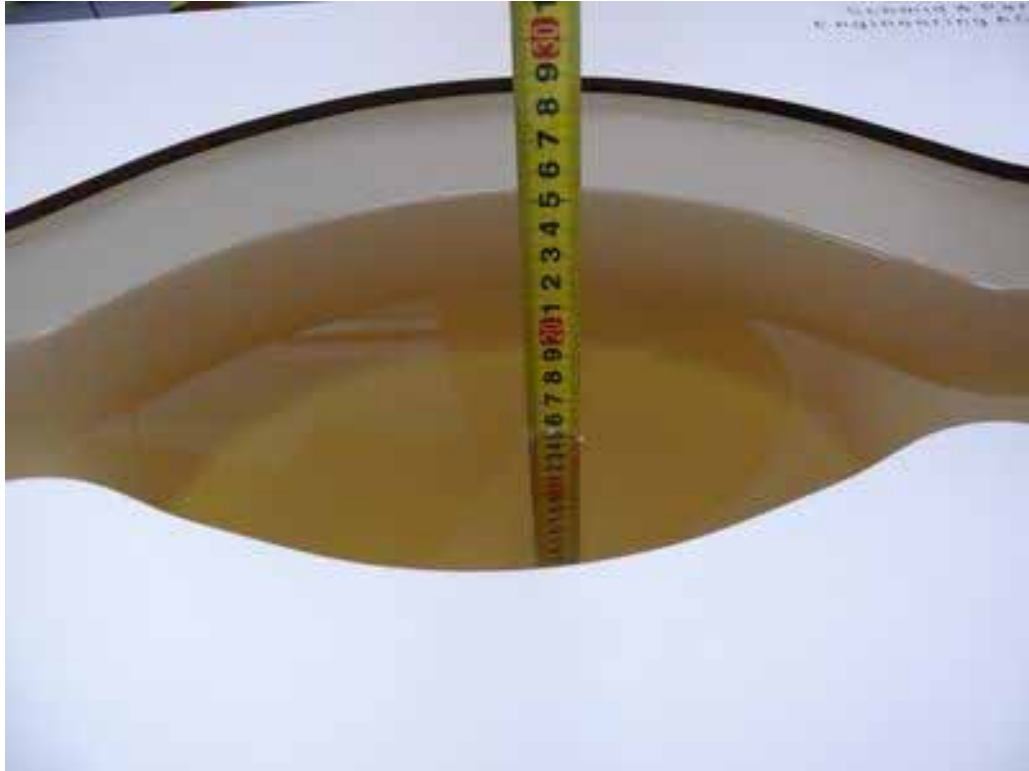
Picture 3: Liquid depth in the Flat Phantom (835 MHz) (15.2cm deep)
