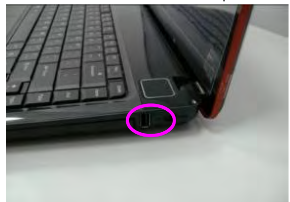
Picture 1-f: Lenovo Y-450 with vertical USB slot
