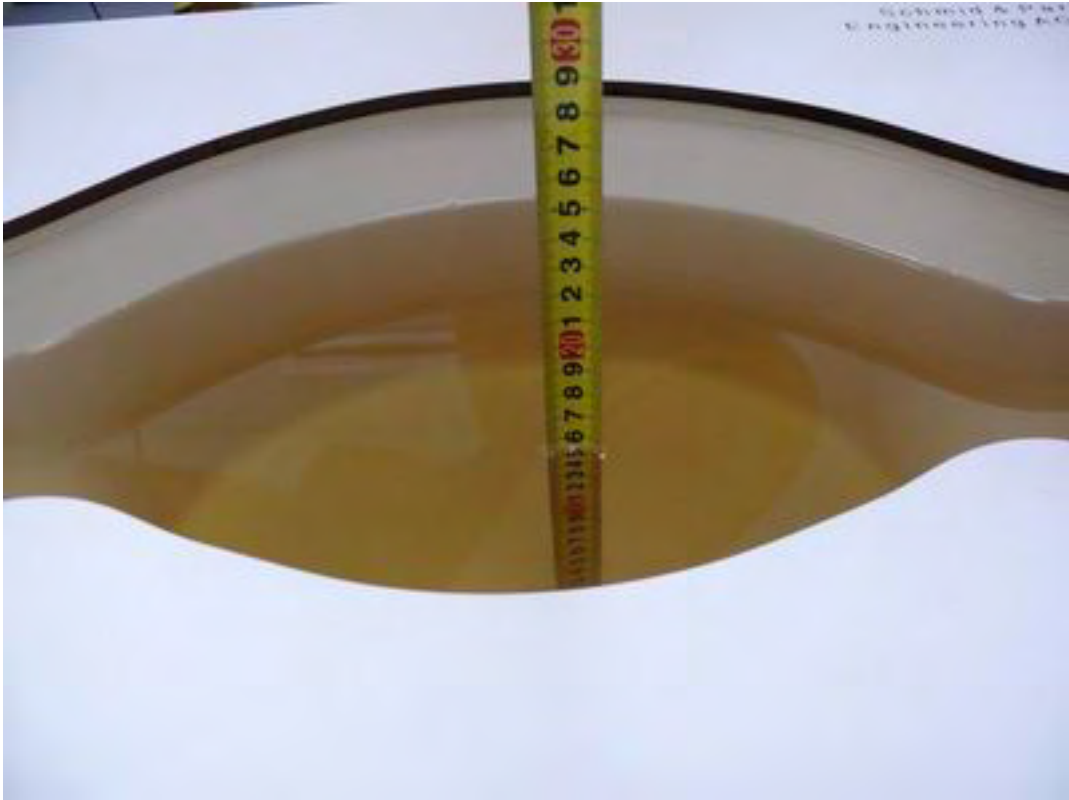
Picture 3: Liquid depth in the Flat Phantom (835 MHz, 15.2cm depth)
