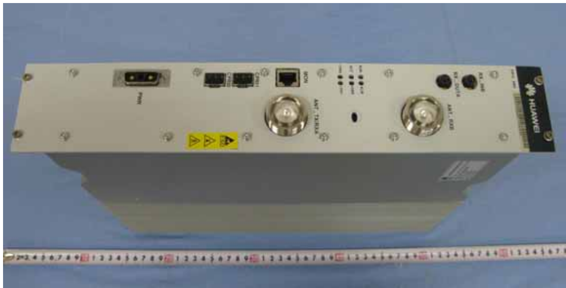
Figure 1, Front view of CRFU-AWS
