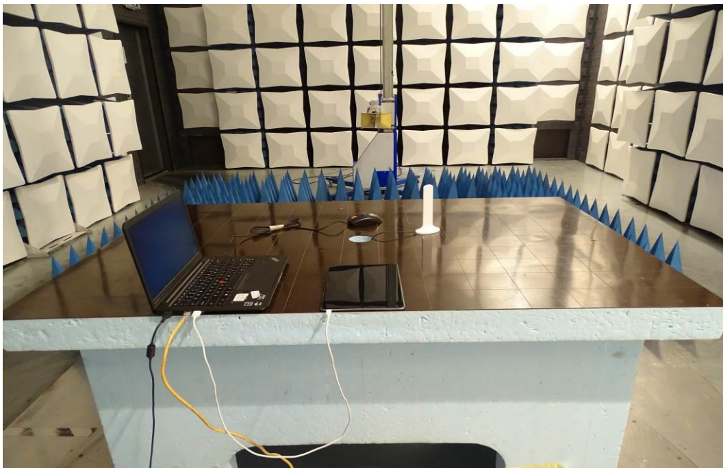
Radiated Disturbance Emissions (1GHz to18GHz)
