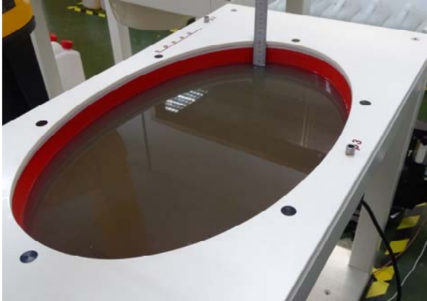
Photo 12: ELI4 Phantom MBBL600-6000MHz Depth (15.1cm)
