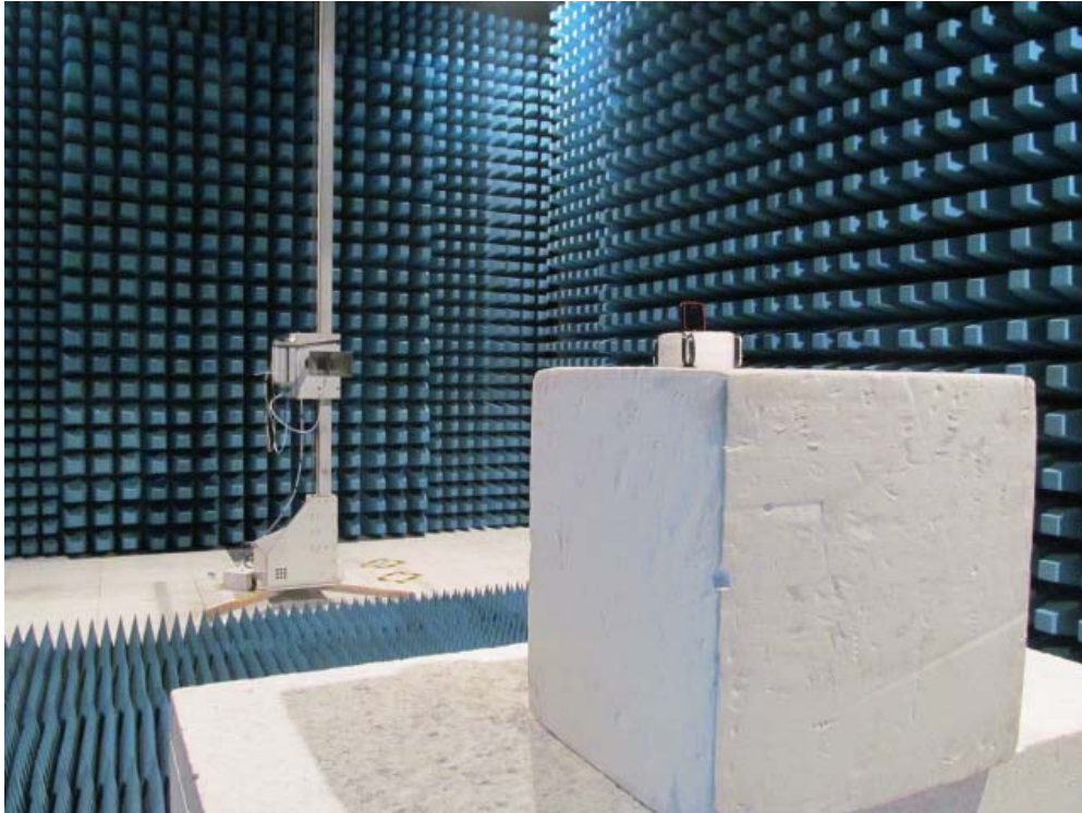
Description: EIRP Test Setup
