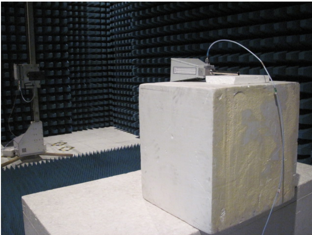
Description: Substitution Antenna for EIRP Test
