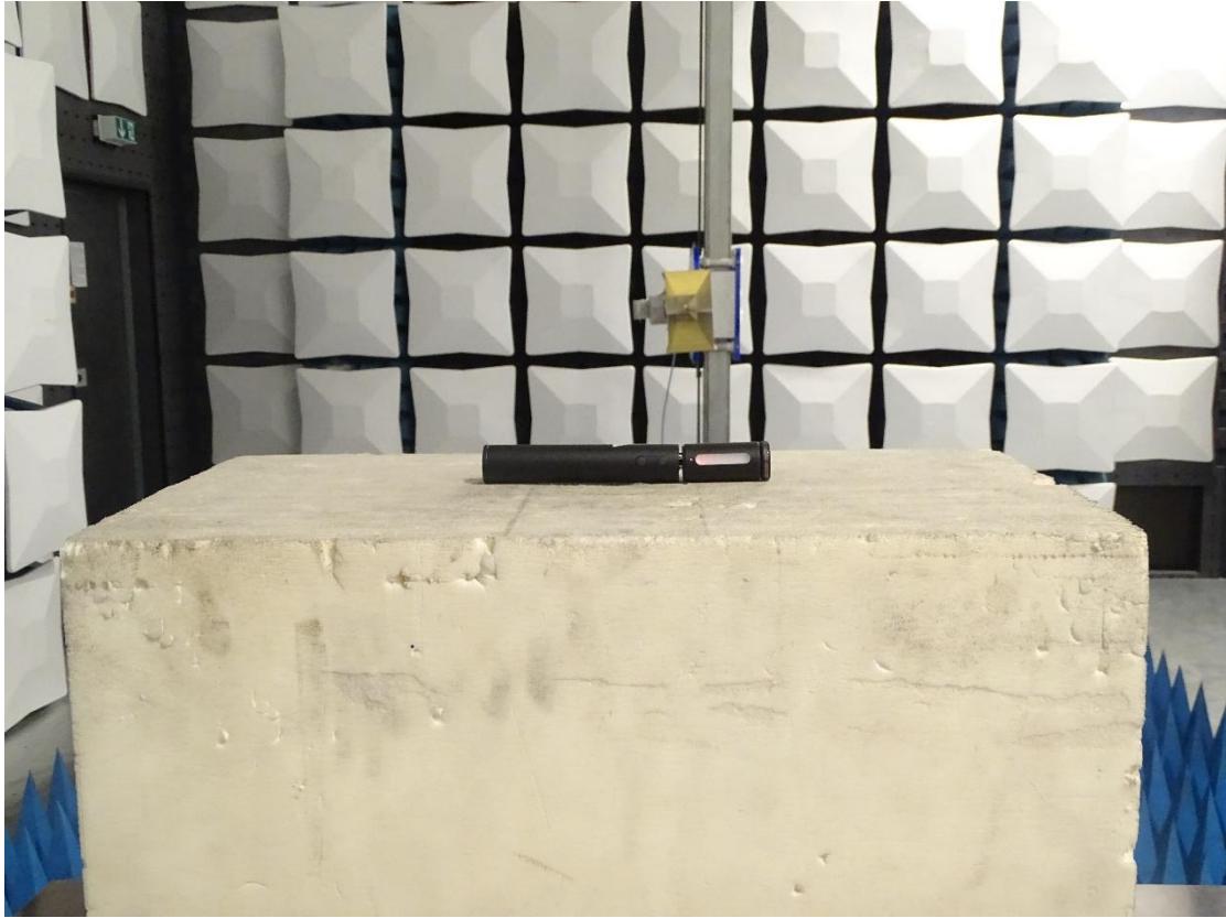
Radiated Spurious Emission (1GHz to18GHz)
