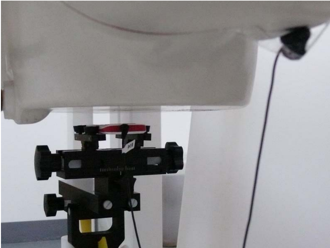
Picture 11: Body with earphone, The EUT display towards ground, the distance from handset to the bottom of the Phantom is 15mm
