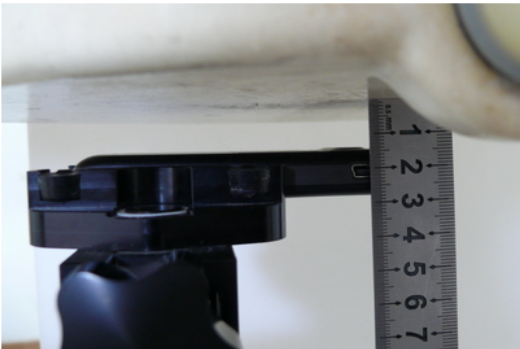
Picture 9 Body, towards the ground, the distance from handset to the bottom of the Phantom is 15mm)
