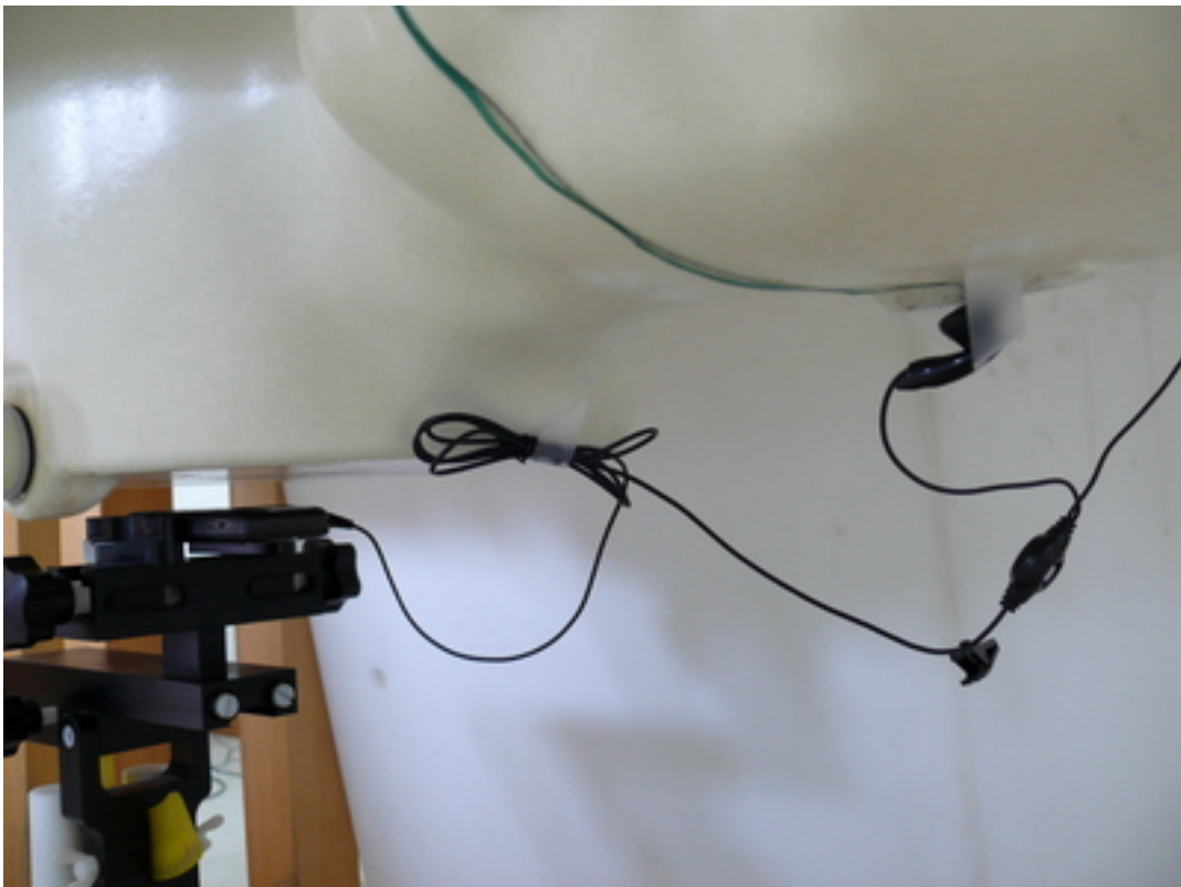
Picture 11 Body with earphone, towards the ground, the distance from handset to the bottom of the Phantom is 15mm)
