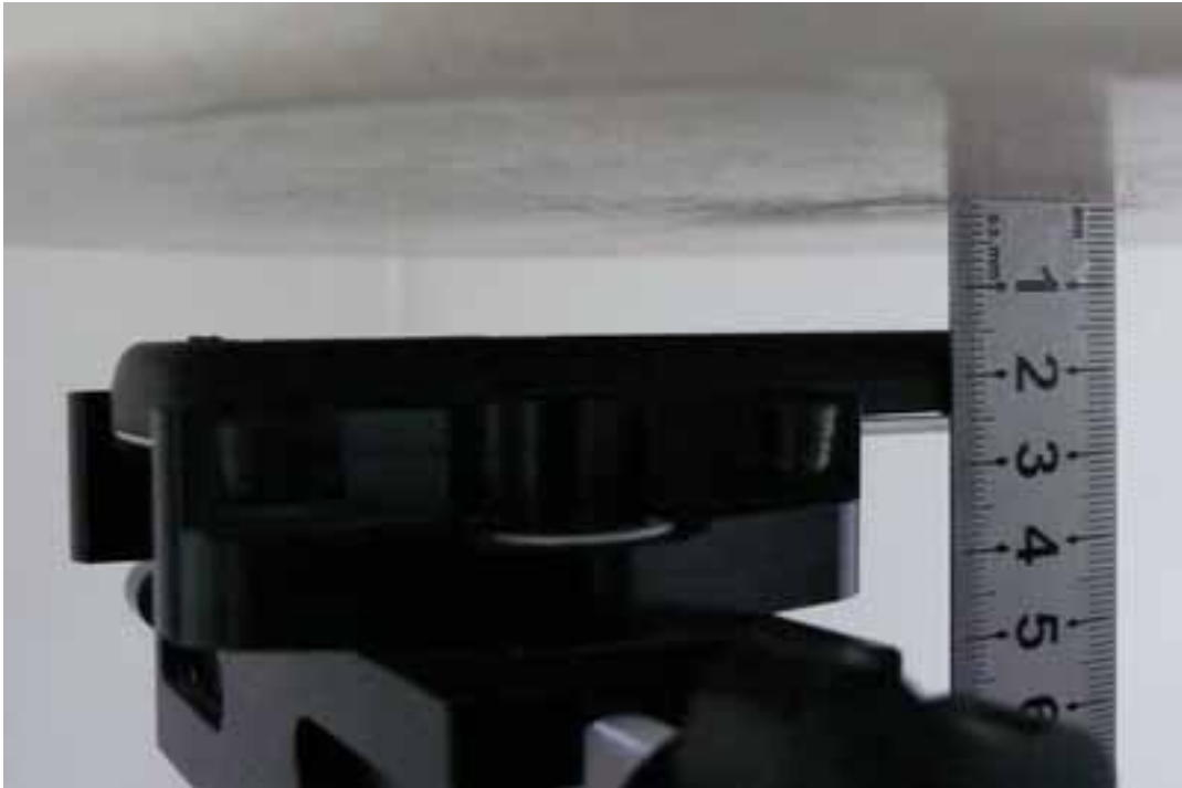
Picture 7: Body, The EUT display towards ground, the distance from handset to the bottom of the Phantom is 15mm)
