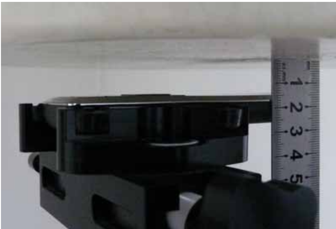
Picture 8: Body, towards phantom, the distance from handset to the bottom of the Phantom is 15mm)
