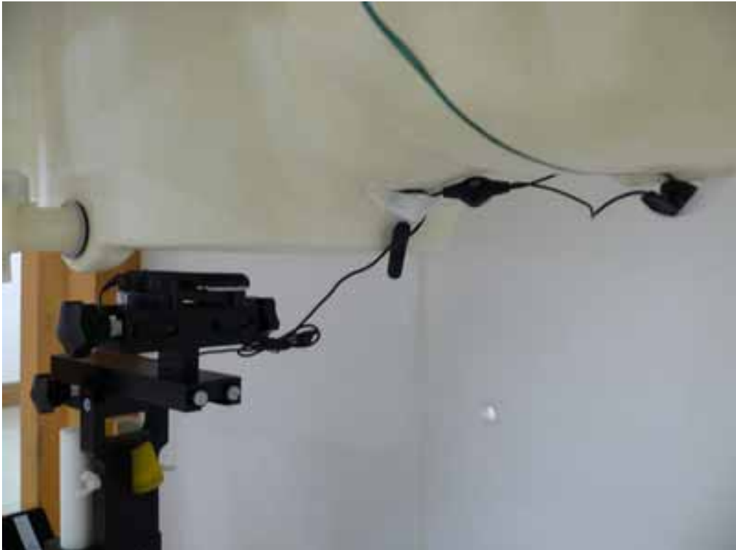
Picture 9: Body with the Earphone, towards ground, the distance from handset to the bottom of the Phantom is 15mm)
