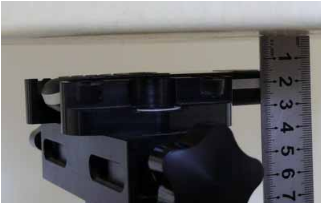
Picture 10: Body, display towards phantom, the distance from handset to the bottom of the Phantom is 15mm)
