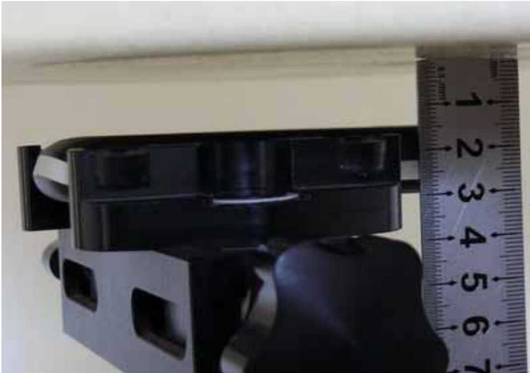
Picture 9: Body, The EUT display towards ground, the distance from handset to the bottom of the Phantom is 15mm)
