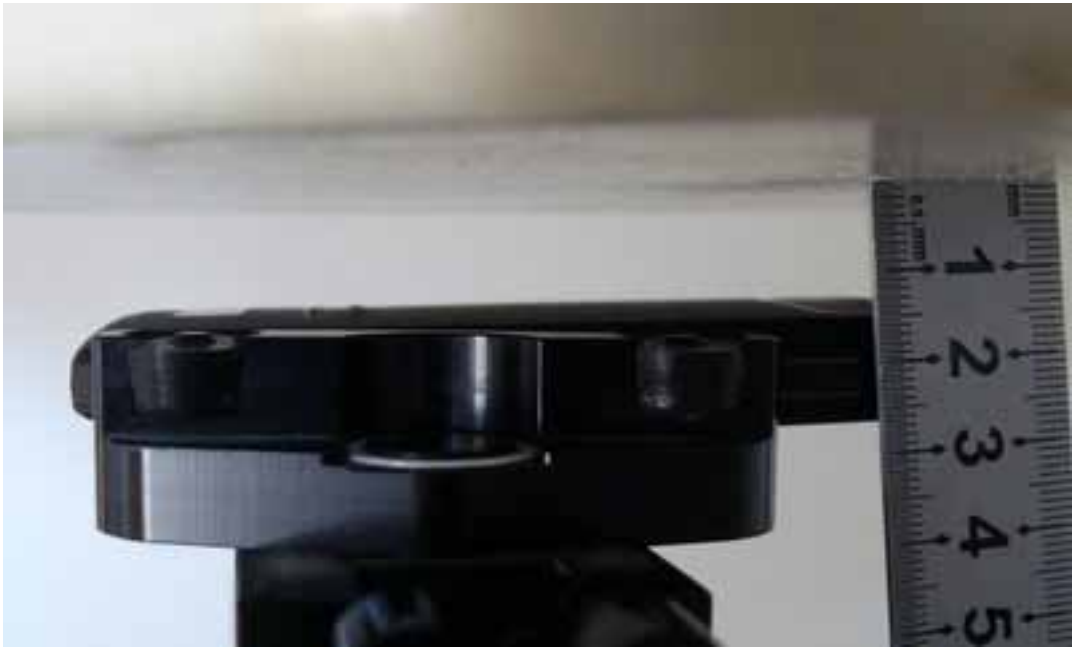
Picture 9: Body, The EUT display towards ground, the distance from handset to the bottom of the Phantom is 15mm)
