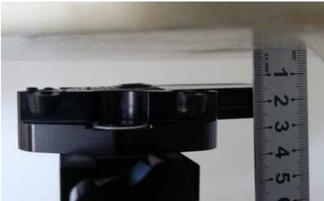
Picture 10: Body, The EUT display towards phantom, the distance from handset to the bottom of the Phantom is 15mm)
