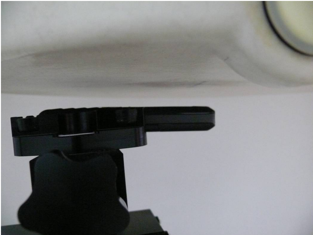
Picture 9: Body, towards the Phantom, the distance from handset to the bottom of the Phantom is 15mm)
