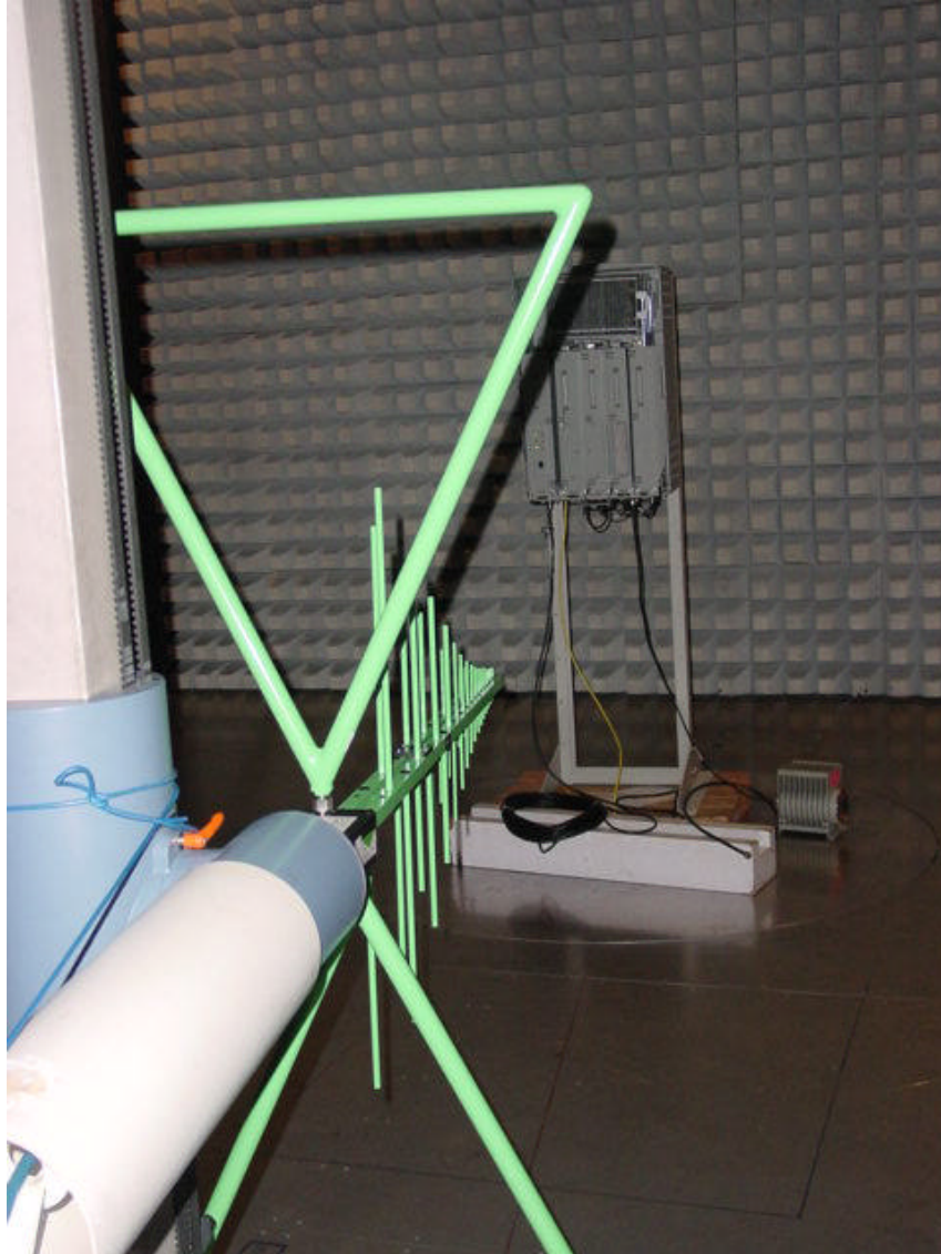
Photo ERP Measurement 30 MHz – 1 GHz
