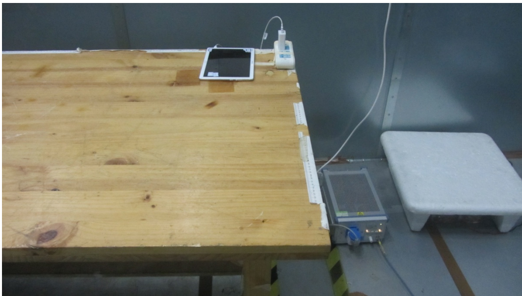
Picture 2 Conducted Emission Test Setup
