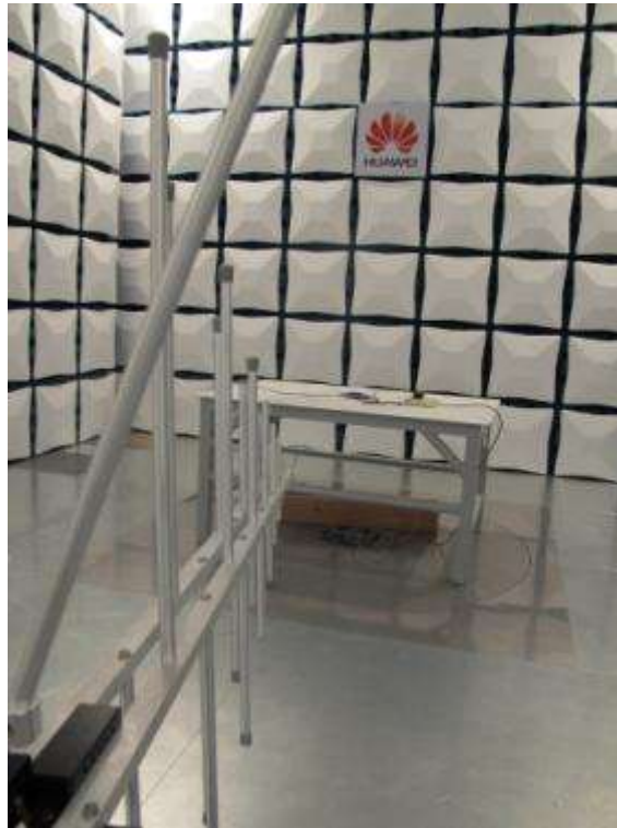
Radiated emission for 30 MHz to 1 GHz of TC/TC2
