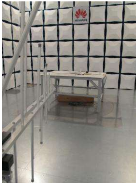
Radiated emission for 30 MHz to 1 GHz of TC3/TC4
