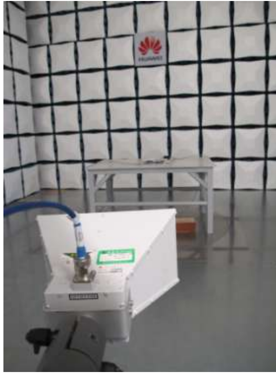
Radiated emission for 1 GHz to 6 GHz of TC1/TC2
