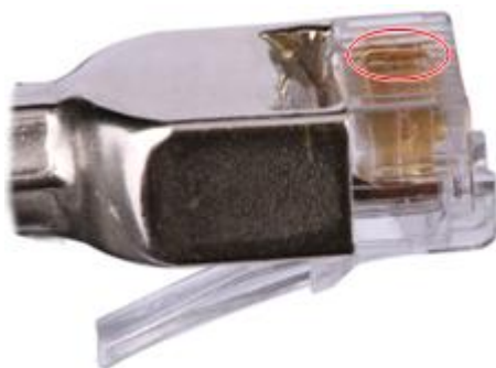
Figure 5-34 Unparallel contact strips of different heights
