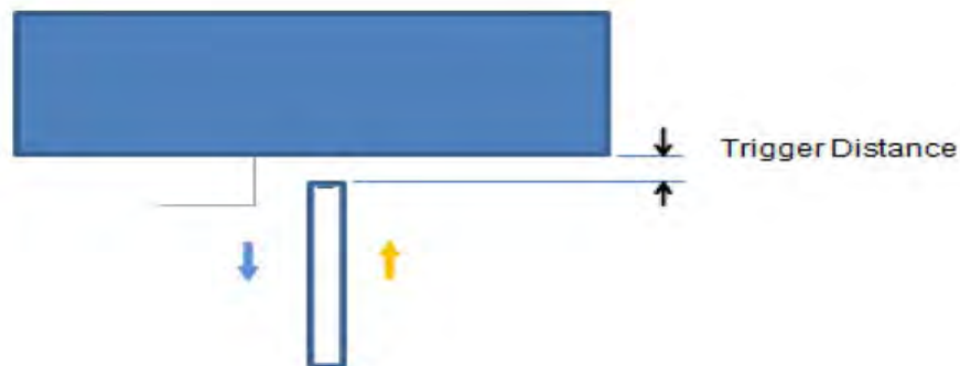
Picture: Proximity sensor triggering distances assessment (Bottomside)
