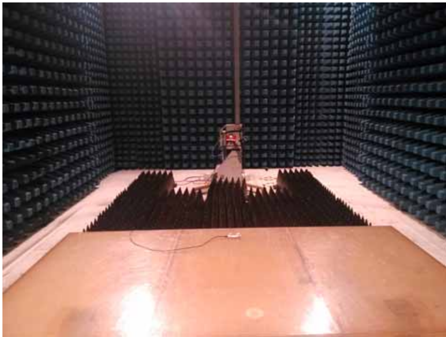
Description: Radiated Emission Test Setup for 1~18GHz
