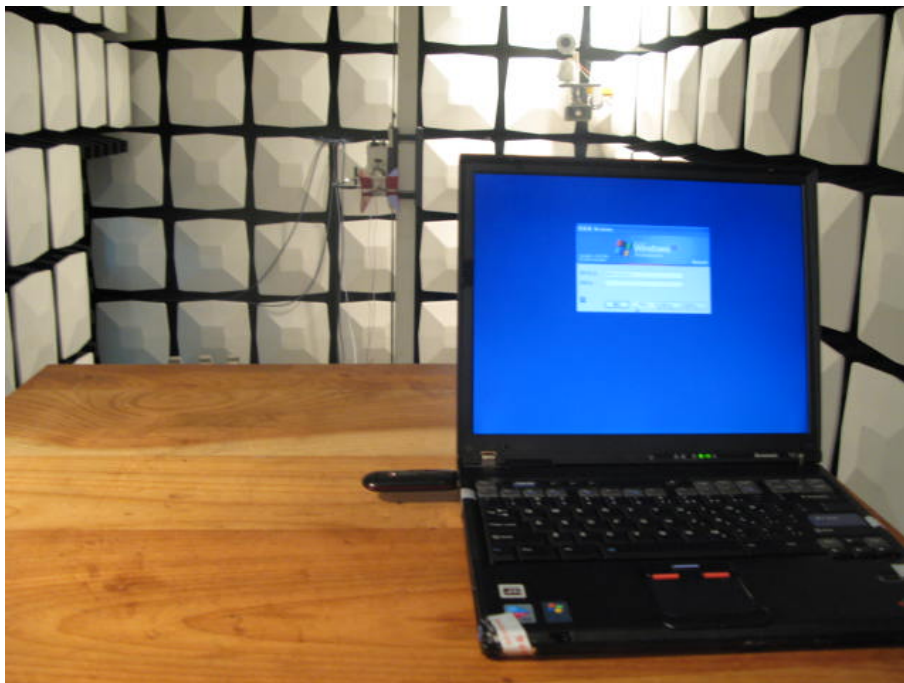
Radiated Spurious Emission (2GHz to 18GHz)
