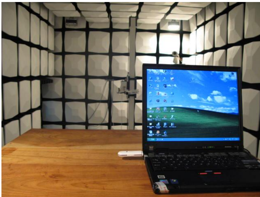
Radiated Spurious Emission 18G~26.5GHz
