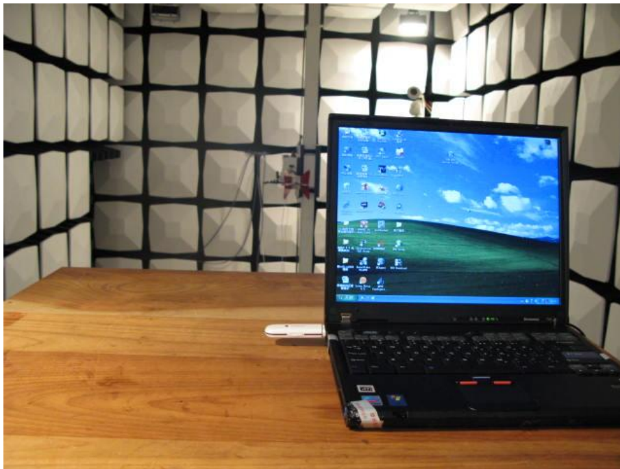
Radiated Spurious Emission (2GHz to18GHz)
