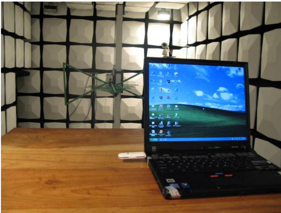
Radiated Spurious Emission (below 2GHz)
