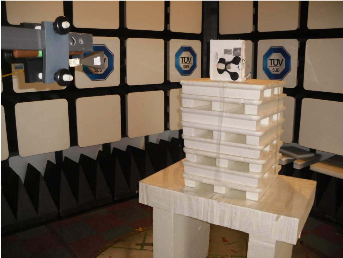
Figure 5 – Radiated Emissions Setup – Photo 3
