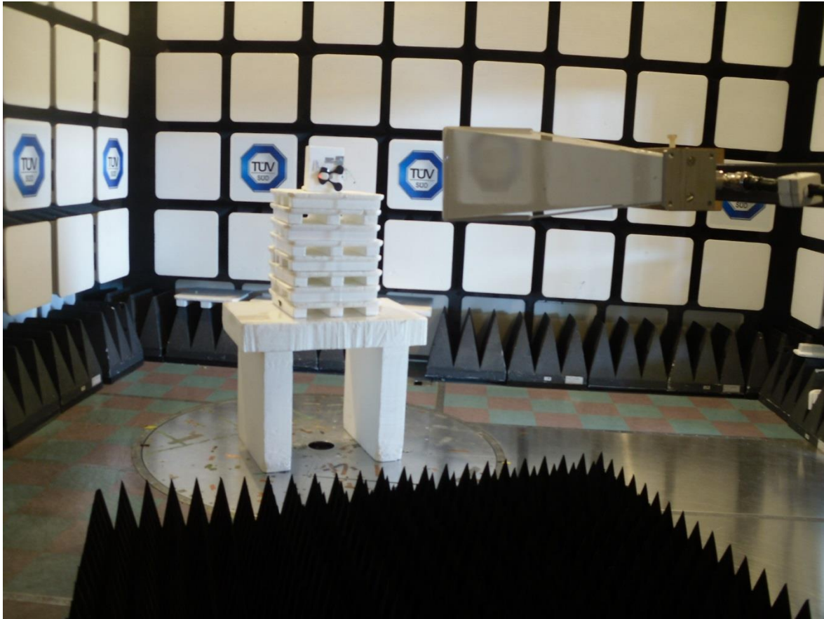
Figure 4 – Radiated Emissions Setup – Photo 3
