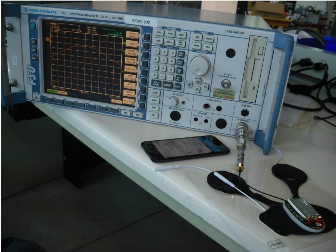
Figure 6 – Antenna Port Conducted Emissions Setup
