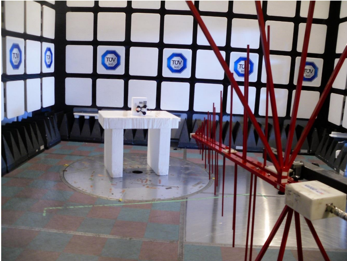
Figure 3 – Radiated Emissions Setup – Photo 2
