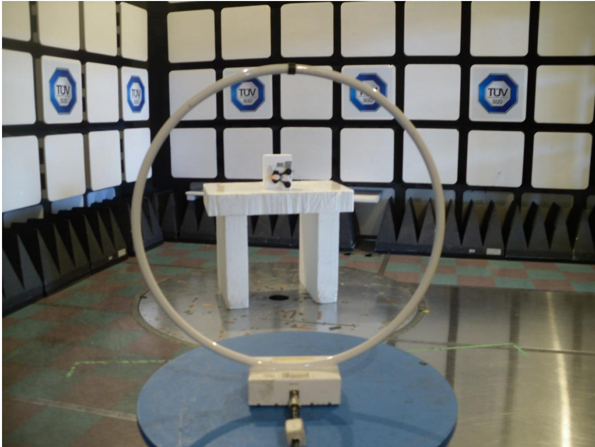
Figure 2 – Radiated Emissions Setup – Photo 1
