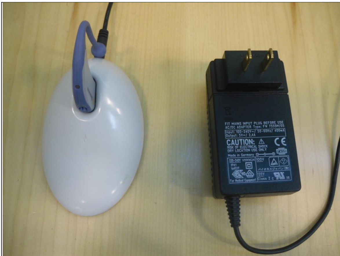
EUT with AC/DC Power supply adaptor
