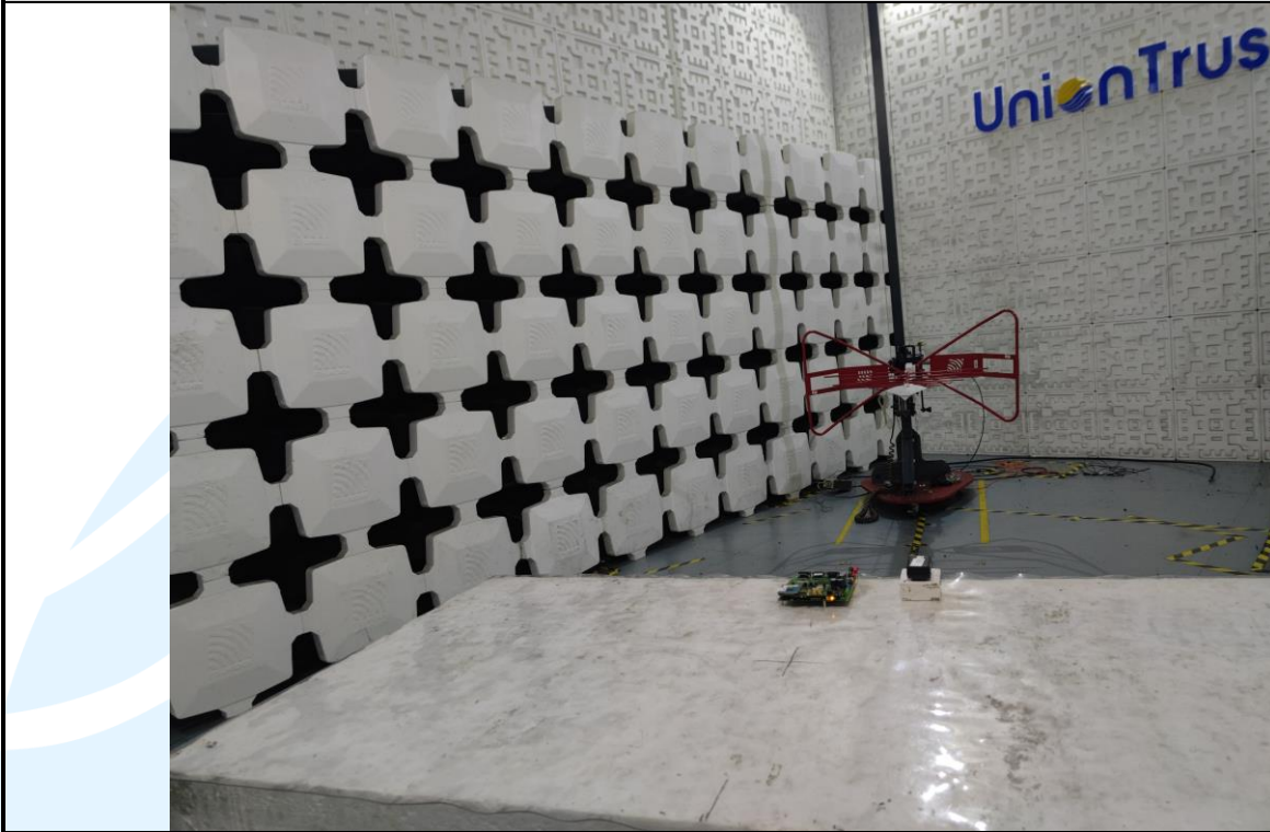
Radiated emission Test Setup-1 (30 MHz~1 GHz)
