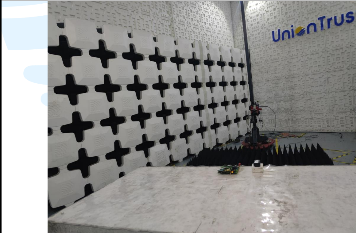
Radiated emission Test Setup-2 (Above 1 GHz)
