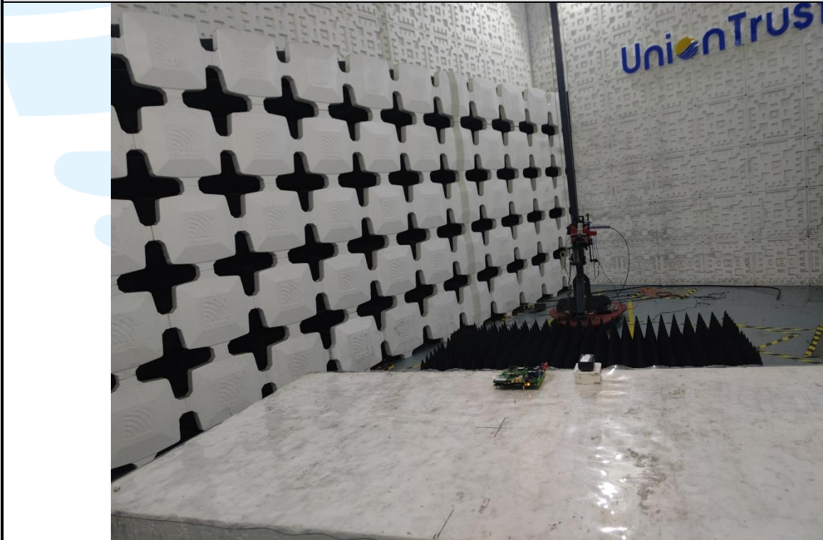
Radiated emission Test Setup-2 (Above 1 GHz)
