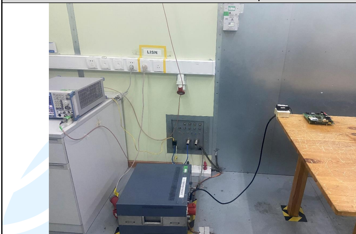
Conducted Emission Test Setup-3
