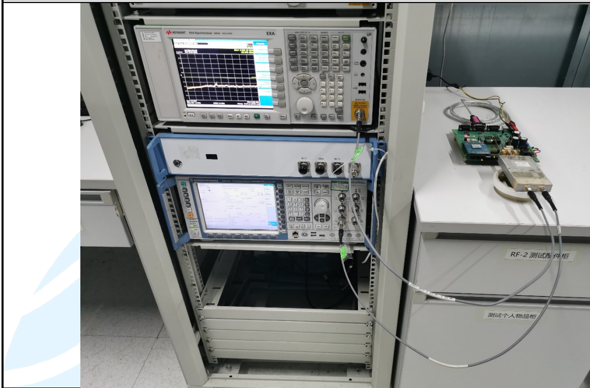
RF Conducted Test Setup
