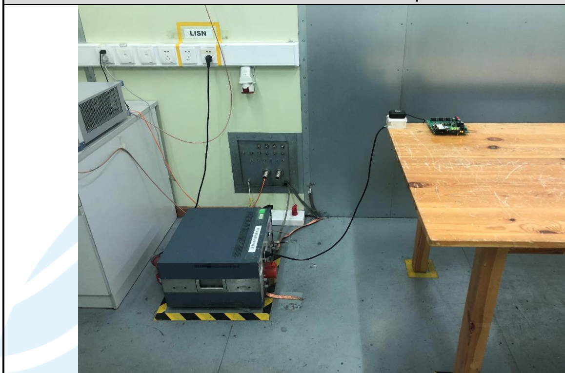
Conducted Emission Test Setup
