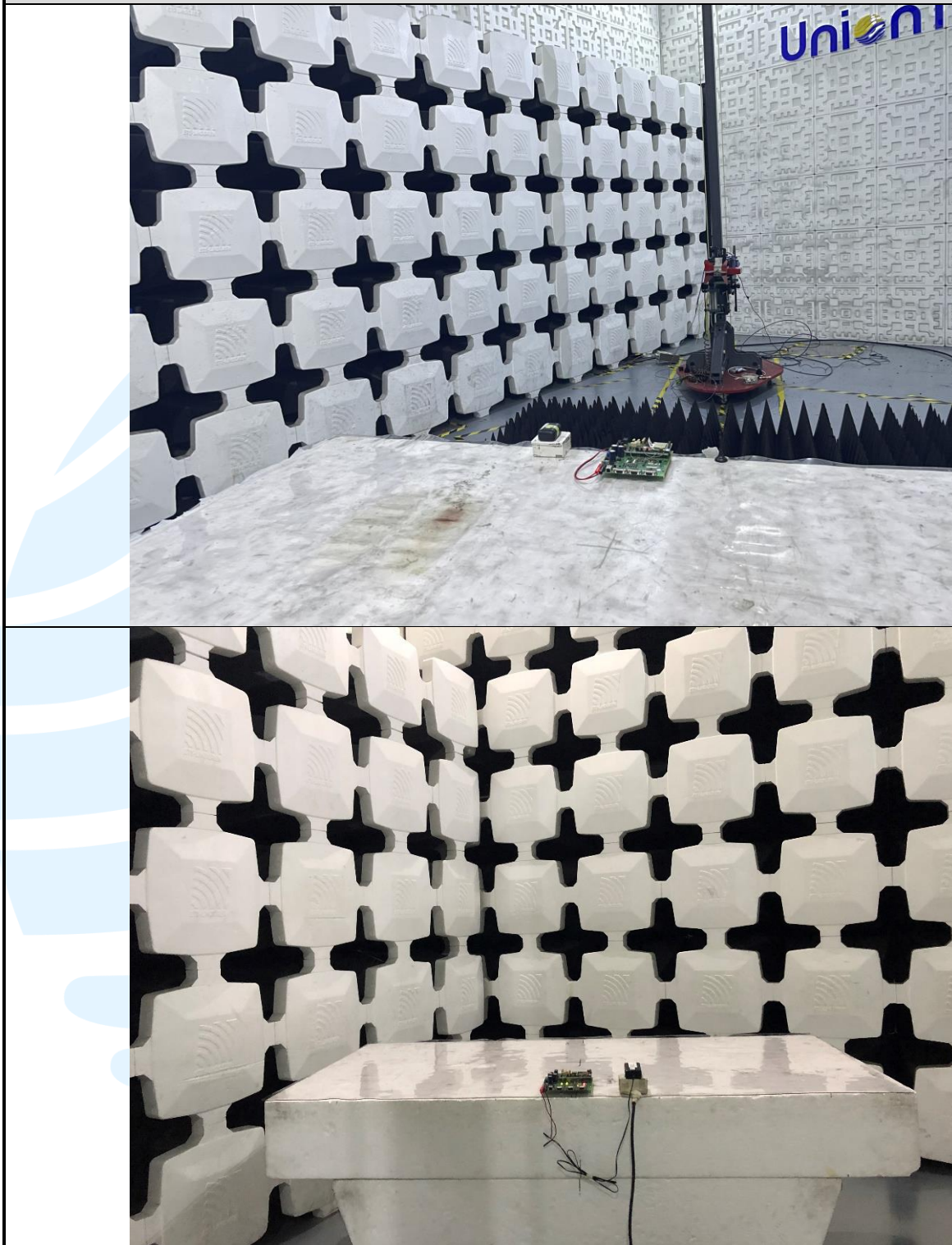
Radiated emission Test Setup-2 (Above 1 GHz)
