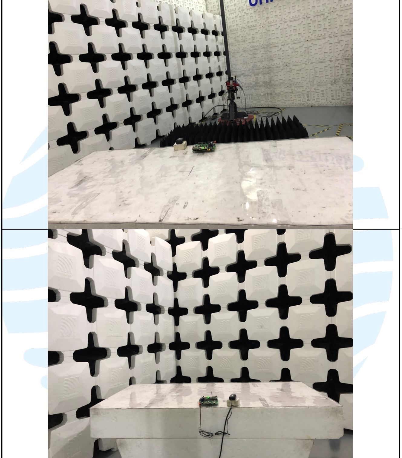
Radiated emission Test Setup-2 (Above 1 GHz)
