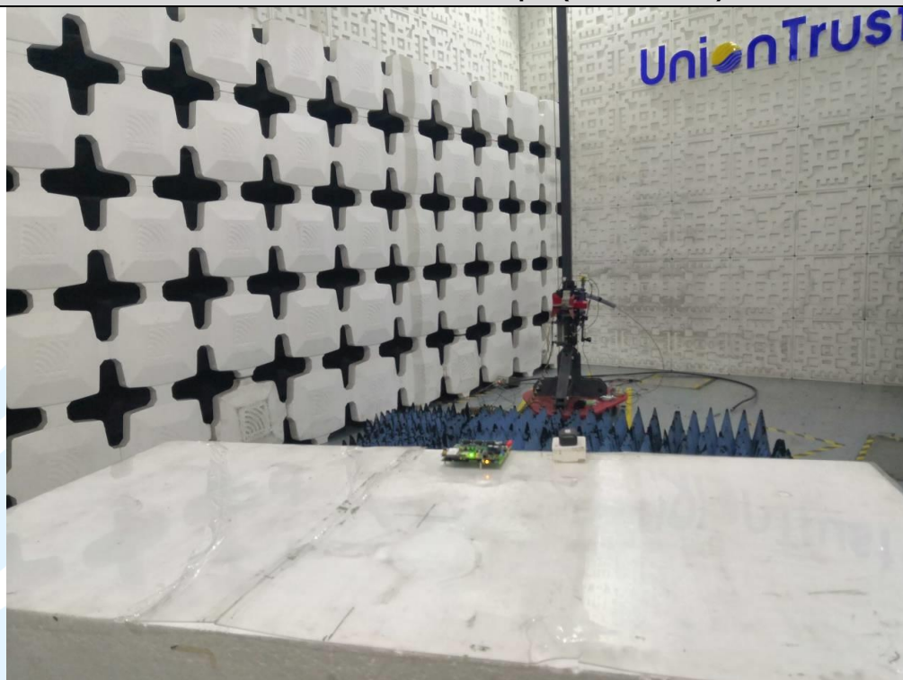
Radiated emission Test Setup-2 (Above 1 GHz)
