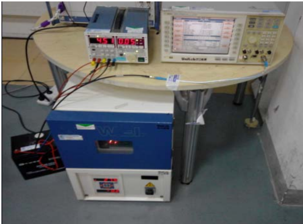
Frequency Stability Under Temperature & Voltage Variations Setup
