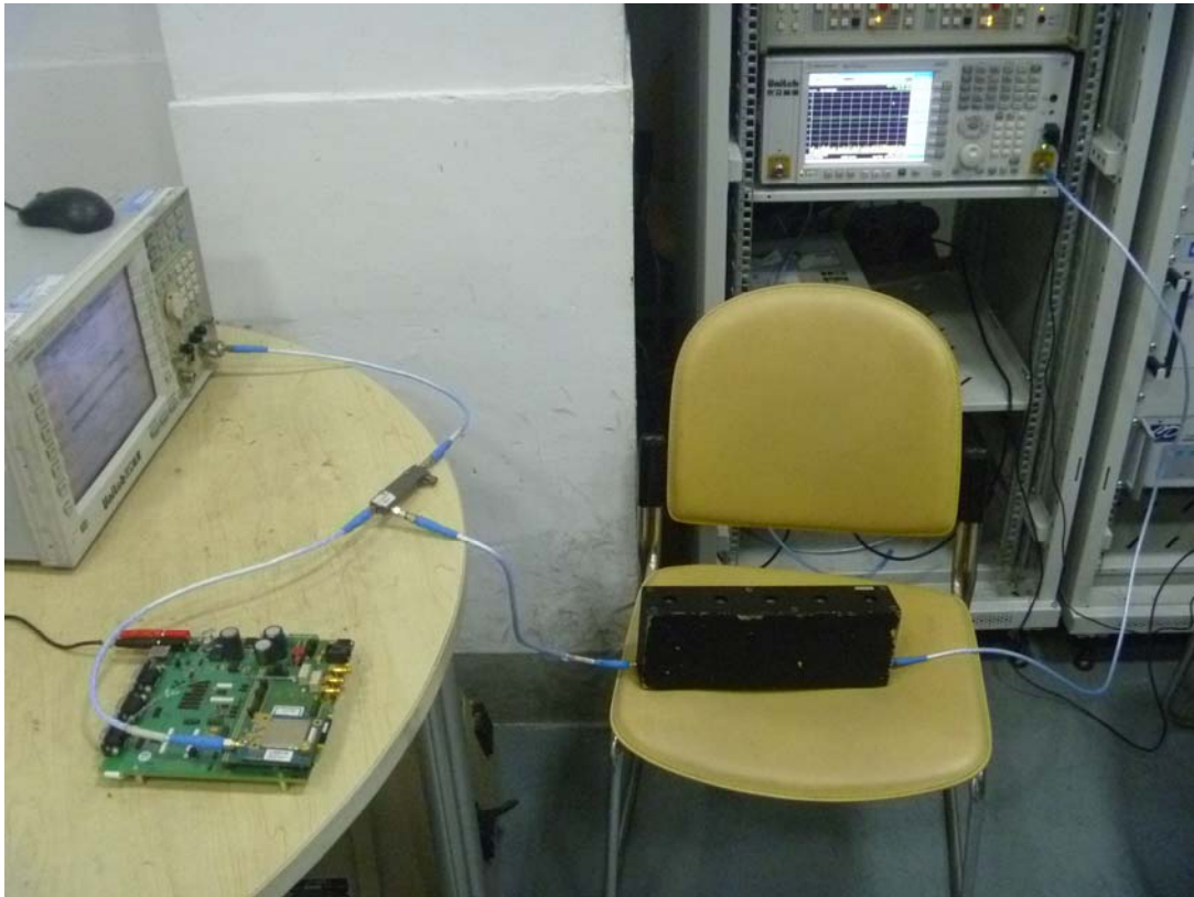
Frequency Stability Under Temperature & Voltage Variations Setup
