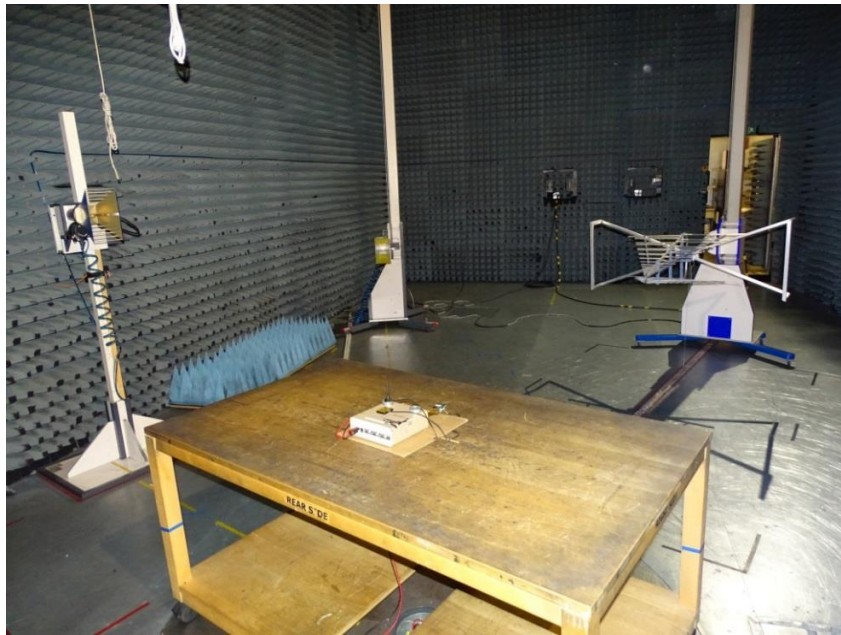
Photo 1: Test setup for radiated measurements below 1 GHz
