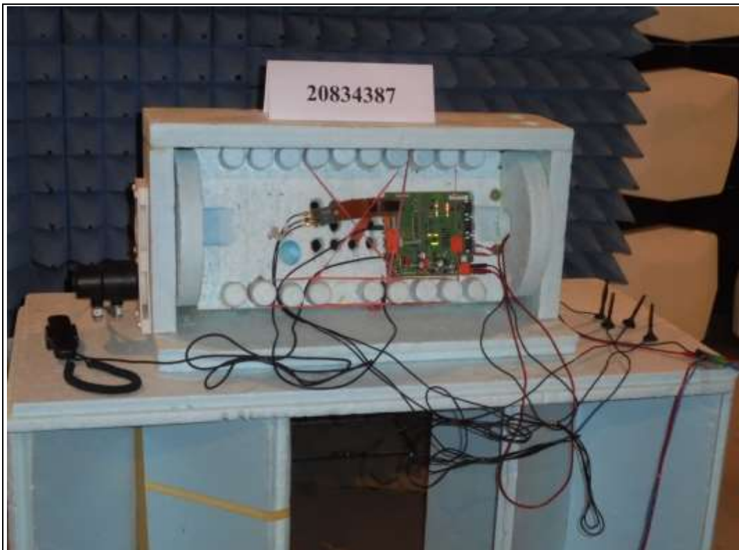
Photograph 2: Radiated measurements test set-up, magnetic field strengths
