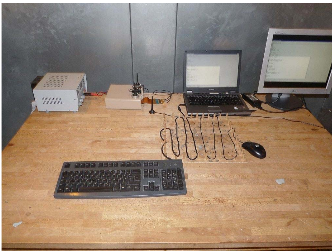
Photo 1: Test setup for conducted measurements (AC Port (power line), EUT supplied by AC/DC Power Supply, intentional / unintentional radiator §15)
