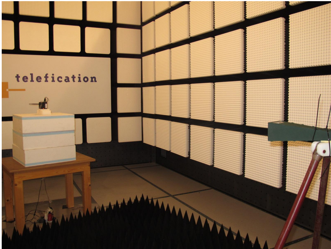
Photograph 4: Radiated emissions test set up, 18 -26 GHz
